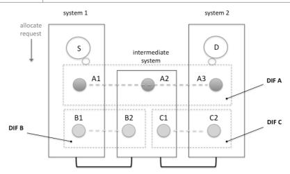
Figure 4 IPC between two application processes in different systems.
